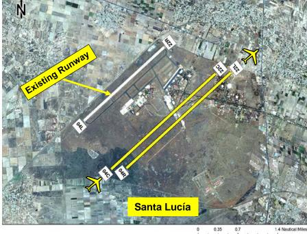
As the 2015 Plan Alternativo did not show parallel runways, MITRE modified them (to ensure parallel runways) to simplify procedure design and air navigation.
